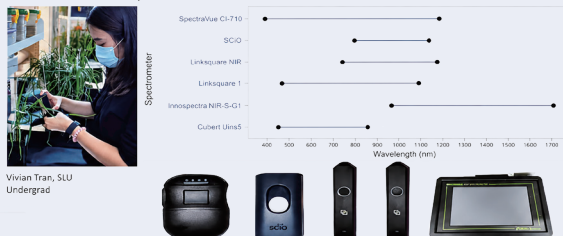
Measuring reflectance on seedlings with handheld spectrometers
